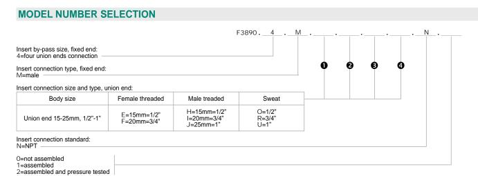
Example: F3890.4.M.H.H.H.H.N.0=By-pass unit, union ends 1/2" NPT male, not assembled.
